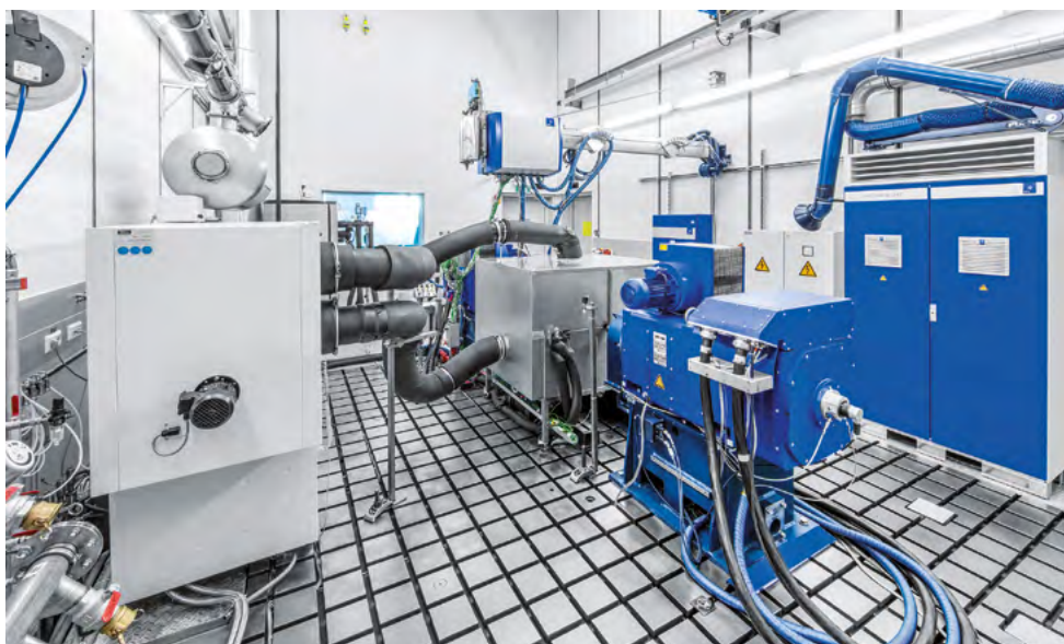
Test bed for electric drives, Photo: AVL List GmbH
